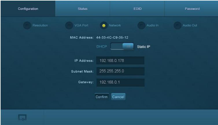
**Figure 4- 6 Configuration-Network**
