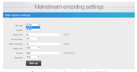
Encoder type: Selector for the type of compression H.264 & H.265
