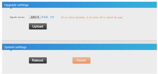
Upgrade setting: Search for software upgrade package and UPLOAD NOTE: CHOOSE THE COMPRESSED UPGRADE PACKAGE(\*.RAR FILE) WITHOUT DECOMPRESSING PACKAGES. DO NOT REFRESH THE PAGE AND OTHER OPERATIONS DURING THE UPGRADE.
