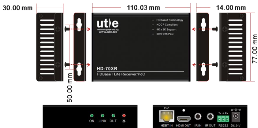
Figure 5-1 Panel drawing of HDMI Twisted Pair PoC Receiver HD-70XR
