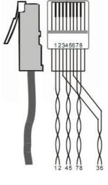
Note: To make a better transmission, cable connectors MUST be metallic, the shielded layer of cable MUST be connected to the connector's metal shell.
