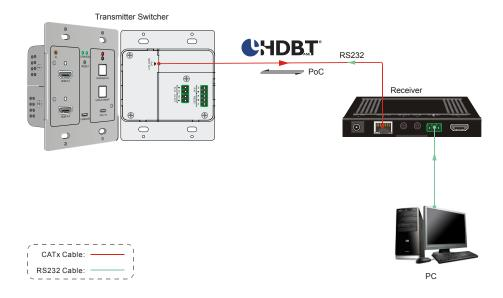
③ To control the far-end third party device, please connect the control device (e.g. PC) to the RS232 port of the switcher, and then please connect the third party device (e.g. projector) to the RS232 port of remote receiver. The connection diagram shown as below:
