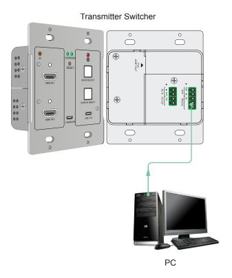
② To control the switcher from remote, please connect a control device (e.g. PC) to the RS232 port of the remote receiver, the connection diagram shown as below:
