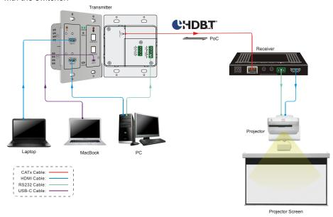
**Note:** We recommend CATx cabling with alien crosstalk prevention technology to ensure the performance of HDBaseT link.
