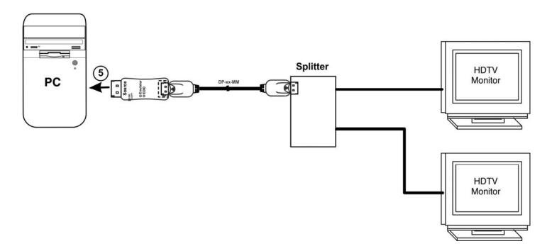
The EDID table copied during the Learning Mode will be available to provide the desired resolution to your monitor(s). Note: Make sure your monitor is capable of displaying the selected resolution.
