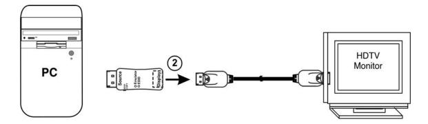
3. Make your connections from the DisplayPort cable to the display, splitter or extender and power the splitter or extender and associated display(s) ON.
