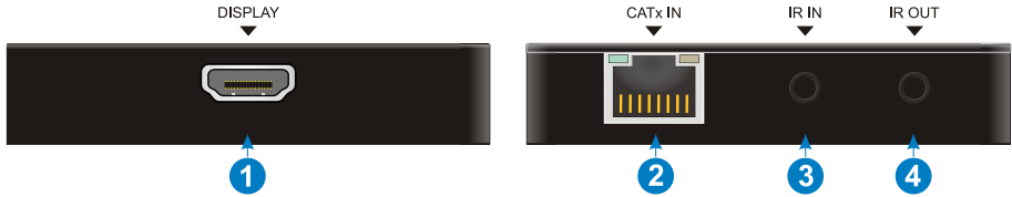
Abbildung 2-2 UHCE-70XLR (4K60 18G HDMI2.0 Receiver)
