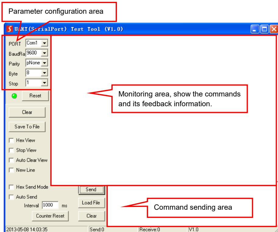
Please set the parameters of COM number, bound rate, data bit, stop bit and the parity bit correctly (Baud rate: 9600 , Data bit: 8 , Stop bit: 1 , Parity bit: none), then the RS232 commands can be sent in Command Sending Area.
