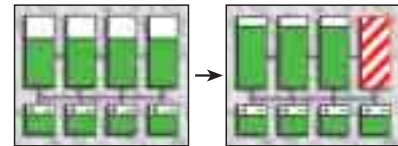
If one board fails, the others share the load. The same principle goes for the batteries.
