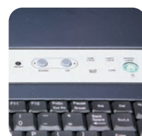
Port Up/ Port Down Switches
